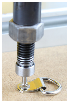
Rivets set flat and smooth both sides
