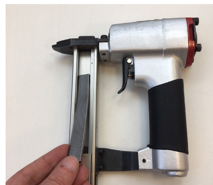
Lay the stick of flexis into the magazine, points down
