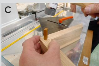
For wider mouldings, using two keys, adjust black plate for position of the first slot and rout all four pieces. Then re-adjust for position of second slot and rout them again.
