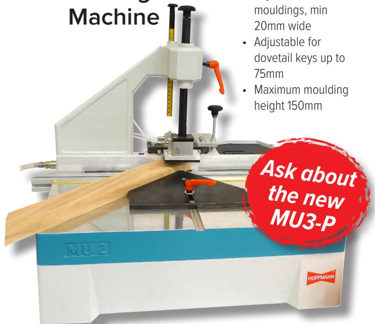
Bench-top machine, for routing a single dovetail slot with each pneumatic machine cycle. Works with Hoffmann Keys W-0, W-1, W-2, W-3 and W-4. Order with W-1 or W-2 router bit, as below.
