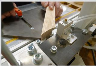
To position the moulding, turn it over, end to end. Line up centre line of slot with indicator and adjust and lock black plate.
