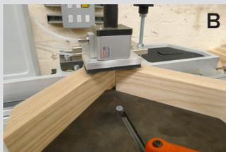
Check slot and adjust setting as required. Then swap position of mouldings and repeat. Do this on each end of all four pieces.
