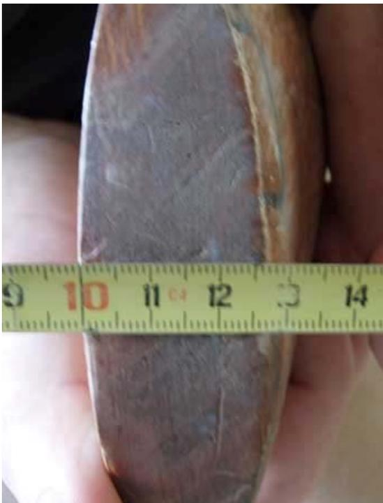
Picture above shows a bat with a toe thickness of 27mm, which is within the normal toe thickness range.
