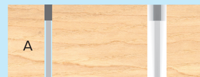
Low vibration - cut is true to kerf High vibration - cut is wider than kerf
